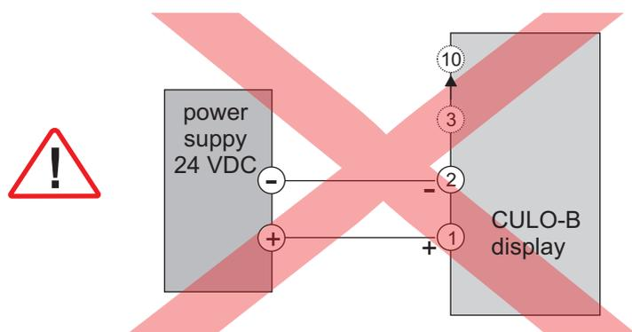
The input 0(4)...20 mA has to be operated with a mA-signal only. A direct connection to a voltage supply (eg 24 VDC) will destroy the indicator and the guarantee does not cover this.
