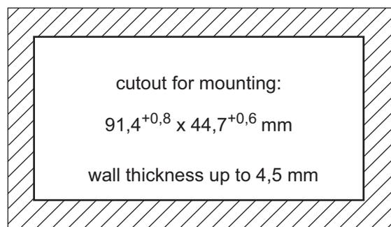
1. Cut the cutout into the control board
