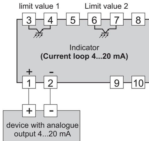
**!** The analogue input of the indicator and the voltage supply are not galvanically insulated.
