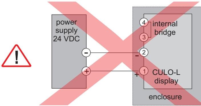
The display is operated in a current loop of 4...20 mA absolutely. A direct connection to a voltage supply (eg 24 VDC) will destroy the indicator and the guarantee does not cover this.
