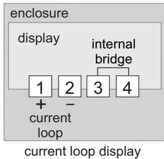
The 4-pole plug-in terminal strip to connect the current loop indicator is at the back of the display and is accessible after the enclosure is opened.
