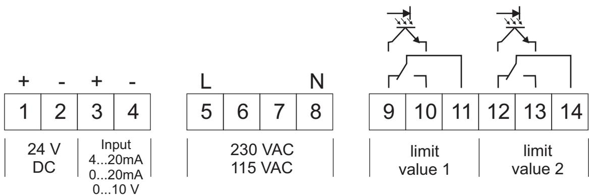
The terminal blocks are located in the bottom of the enclosure
