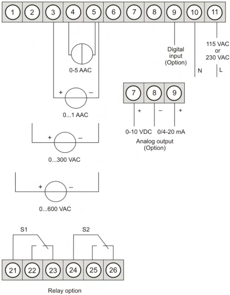
**M2 with digital input and external voltage supply source**
