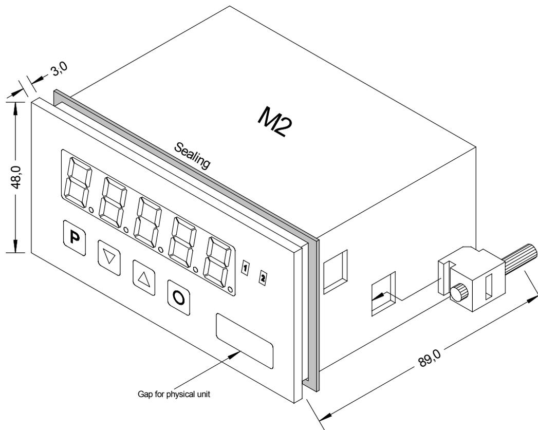
1. After removing the fixing elements, insert the device.
