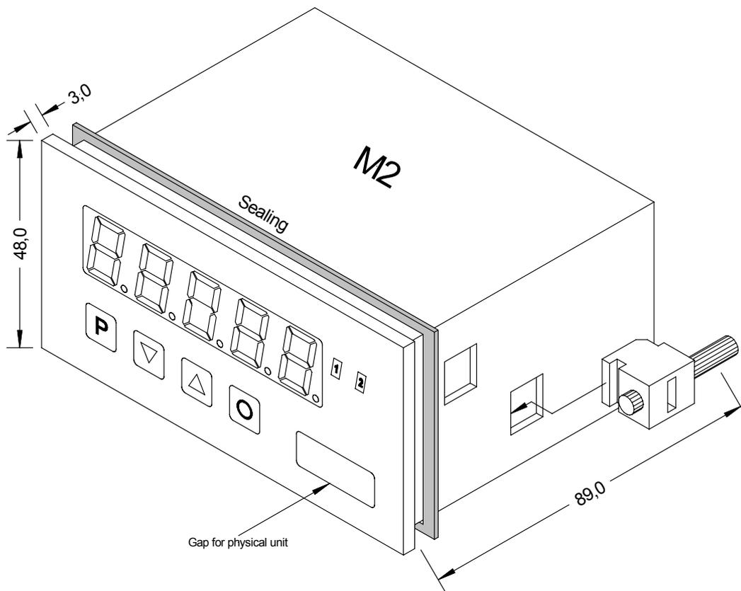
1. After removing the fixing elements, insert the device.
