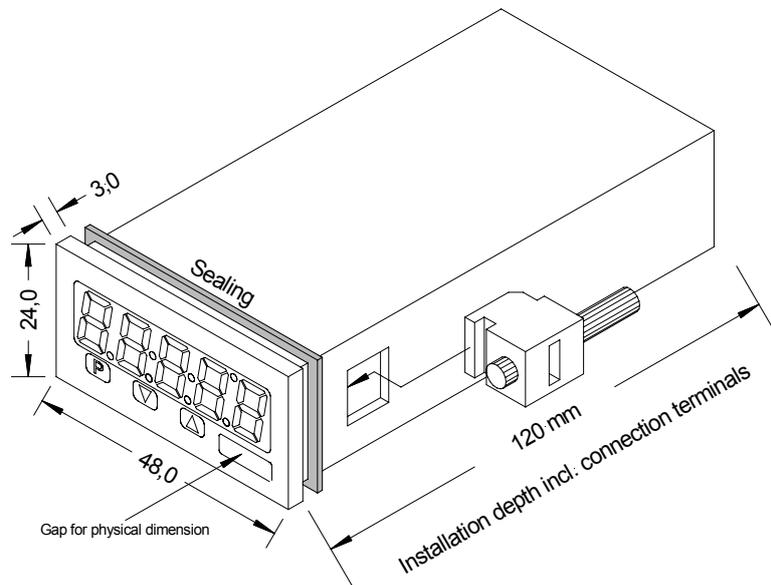
1. After removing the fixing elements, insert the device.
