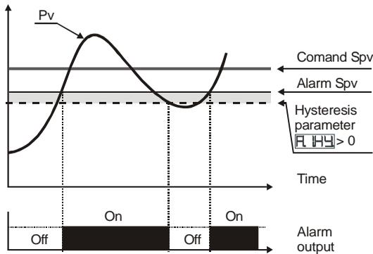
Upper deviation alarm value of alarm setpoint less than “0” and hysteresis value greater than “0” (Par.28  $\text{R.149} > 0$ ).
