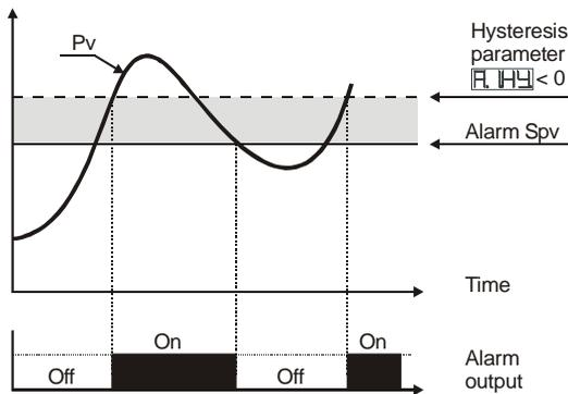
Absolute alarm with controller in heating functioning (Par.11  $\boxed{ACEE}$  selected  $\boxed{HEAT}$ ) and hysteresis value less than "0" (Par.28  $\boxed{A HY} < 0$ ).
