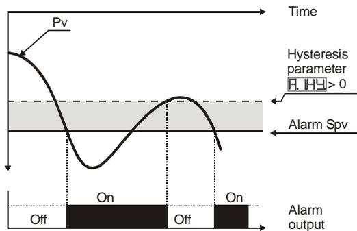
Absolute alarm with controller in cooling functioning (Par.11  $\boxed{ACEE}$  selected  $\boxed{COOL}$ ) and hysteresis value greater than "0" (Par.28  $\boxed{A HY} > 0$ ).
