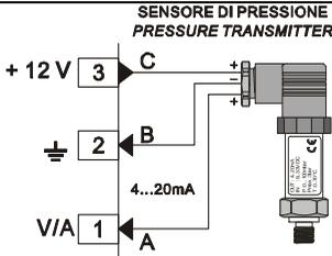
For signals 0/4...20mA with **three-wire sensor**
