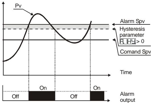
Upper deviation alarm value of alarm setpoint greater than “0” and hysteresis value greater than “0” (Par.28  $\text{R.149} > 0$ ).
