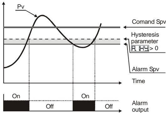
Lower deviation alarm value of alarm setpoint greater than "0" and hysteresis value greater than "0" (Par.28  $\overline{HdAL} > 0$ ).
