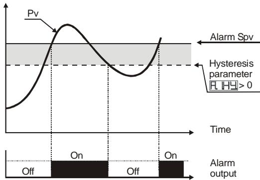
Absolute alarm with controller in heating functioning (Par.11  $\boxed{ACEE}$  selected  $\boxed{HEAT}$ ) and hysteresis value greater than "0" (Par.28  $\boxed{A HY} > 0$ ).
