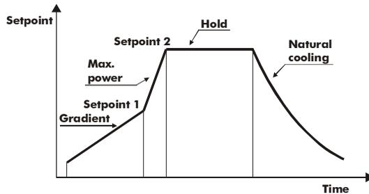
The cycle starts at each activation of the controller, or via digital input if it is enabled for this type of functioning (see parameter 61 `dCt`).
