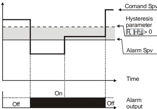
Absolute alarm refers to the command set, with the controller in heating functioning (Par.11 **A.C.E.E.** selected **HEAT**) and hysteresis value greater than "0" (Par.28 **A.HY** > 0).
