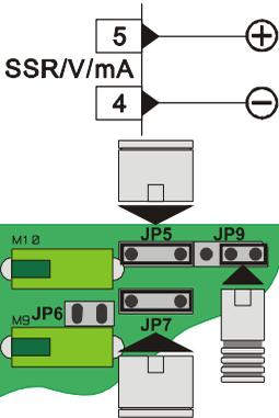
Linear output in **mA** configurable using parameters as command (Parameter `COU`) or retransmission of process-setpoint (Parameter `RETR.`)
