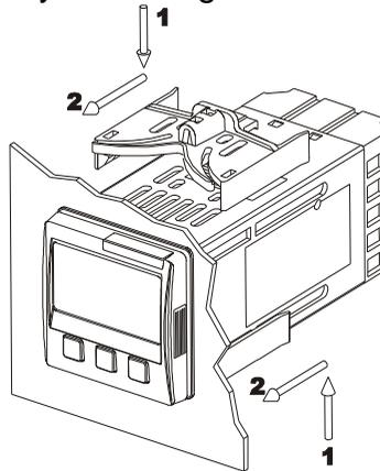
To dismantle, use a screwdriver and slightly force the fixing hooks to remove them from the fixing guide.
