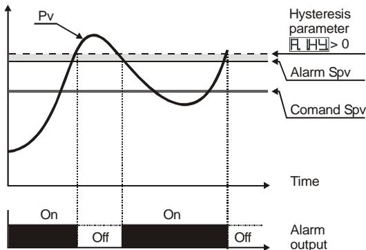
Lower deviation alarm value of alarm setpoint less than "0" and hysteresis value greater than "0" (Par.28  $\overline{HdAL} > 0$ ).
