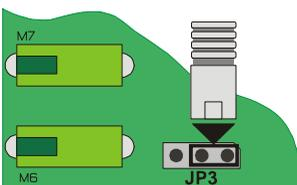
**!** If jumpers are not properly selected, 12Vdc are not available on terminal 3 to power the sensor.
