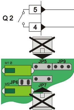
Capacity 5A/250V~ for resistive loads
