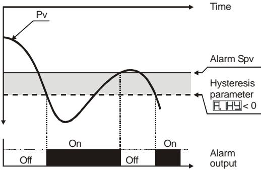
Absolute alarm with controller in cooling functioning (Par.11 **A.C.E.E.** selected **COOL**) and hysteresis value less than "0" (Par.28 **A.HY** < 0).
