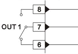
Capacity 5A/250V~ for resistive loads
