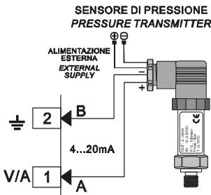
For signals 0/4...20mA with **external power of sensor**
