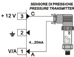
For signals 0/4...20mA with **two-wire sensor**
