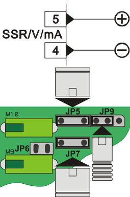
Linear output in **Volt** configurable using parameters as command (Parameter `COU`) or retransmission of process-setpoint (Parameter `RETR.`)
