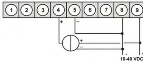
MB2-2V-devices in combination with a 3-wire-sensor 0-10 V
