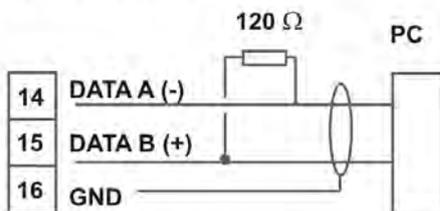
The interface **RS485** is connected via a screened data line with twisted wires (Twisted-Pair). On each end of the bus segment a termination of the bus lines needs to be connected. This is necessary to ensure a secure data transfer to the bus. For this a resistance (120 Ohm) is interposed between the lines Data B (+) and Data A (-).
