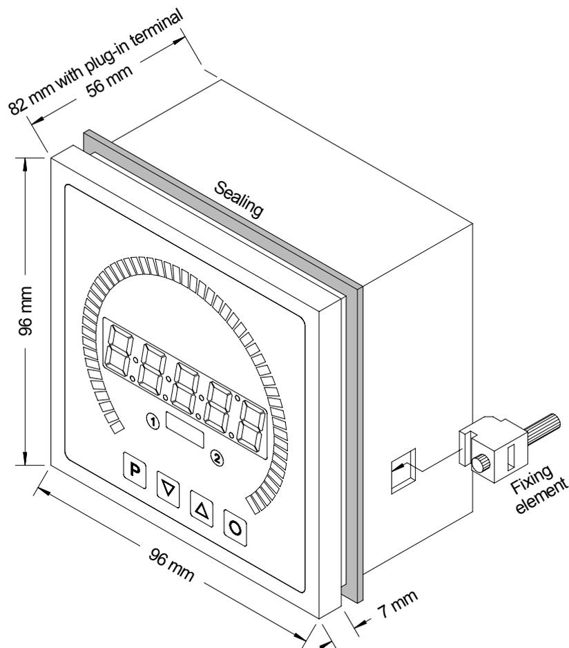
1. After removing the fixing elements, insert the device.
