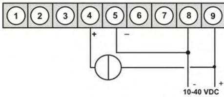
MB2-2V-devices in combination with a 3-wire-sensor 0/4-20 mA
