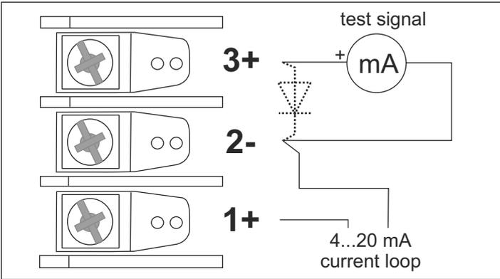
The 4...20 mA test can be measured without interruption of the low-potential circuit between terminal 3(+) and terminal 2(-). The output current is measured with an ammeter for mA across a diode in the output circuit.
