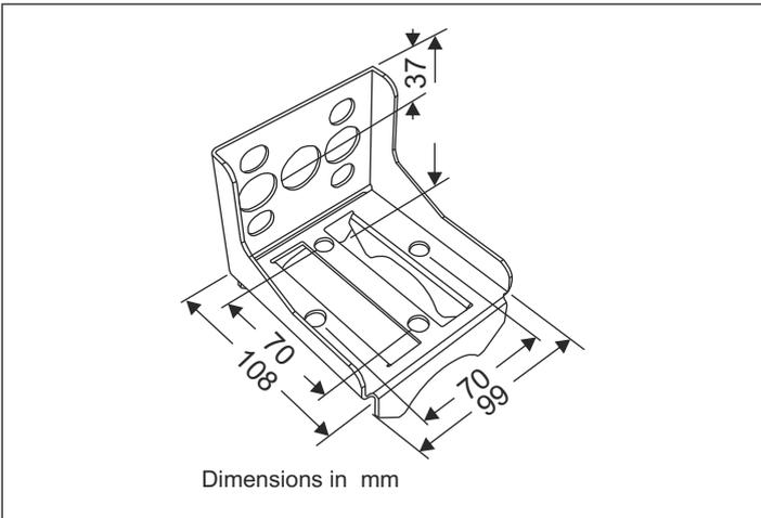
Holder made of steel (zinc coated) for mounting the device on walls or tubes is supplied with the device.
