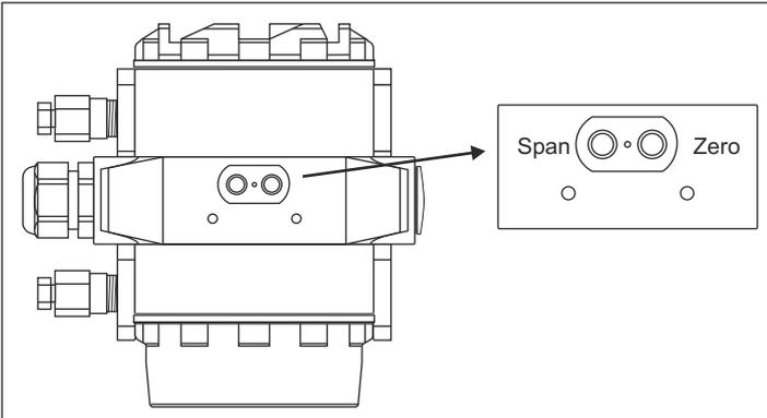
Below the type plate there are 2 key button for easy configuration of zero and span. The keys are Hall effect devices and are completely separated from other parts of the enclosure.
