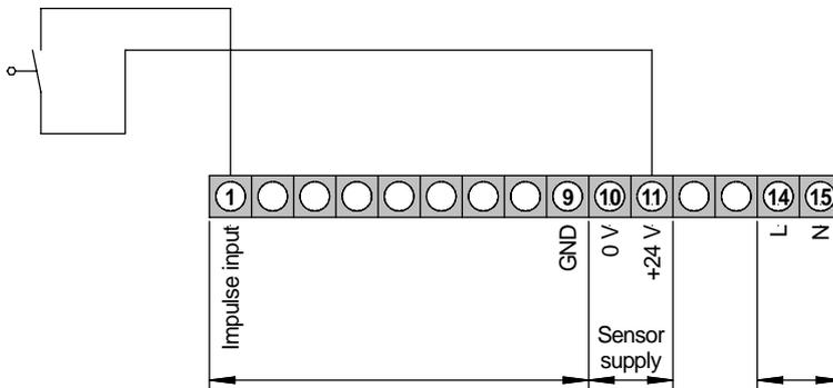
With 115 or 230 VAC supply, the optional sensor supply can be used to feed the sensor.
