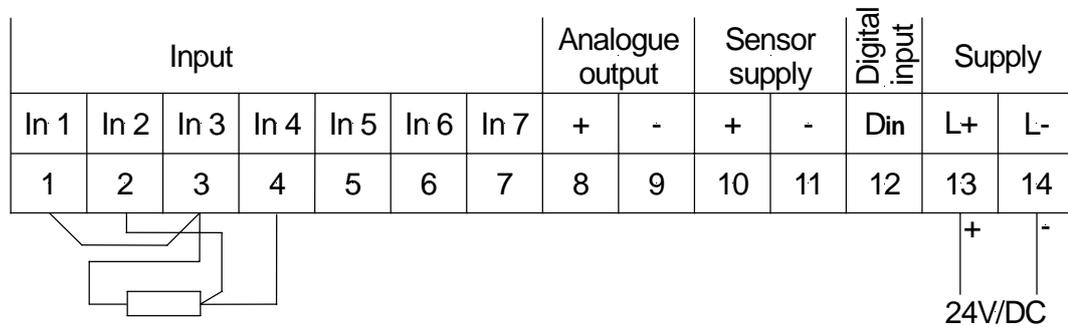
Measurement of a resistance thermometer (e.g. PT100) or resistance in the 4-wire technology; supply voltage 24 VAC
