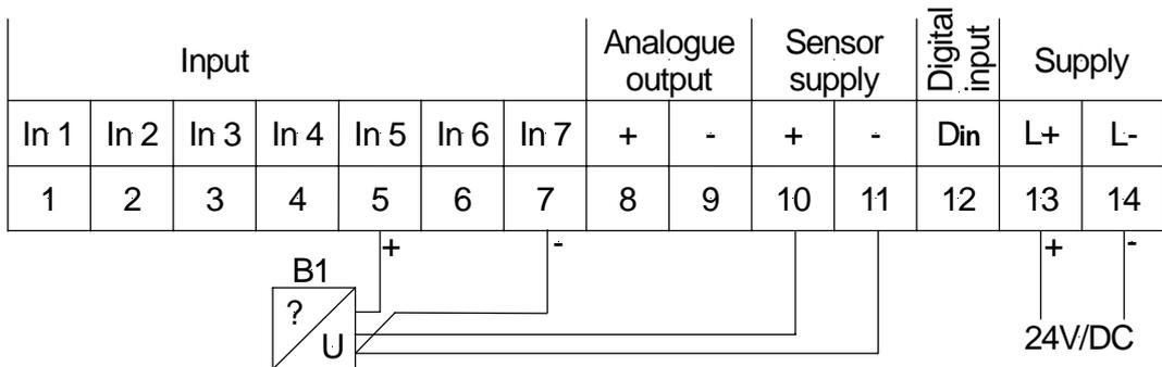
Measurement of a voltage signal ( $\leq 2.5$  V) from a 3-wire transmitter using the sensor supply; supply voltage 230 VAC
