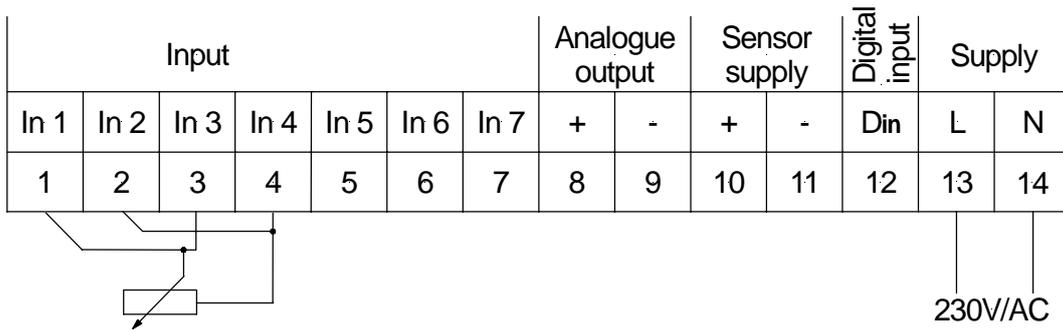
Measurement of a thermocouple; connection of the analogue output; connection of the digital input to the sensor supply; supply voltage 230 VAC.
