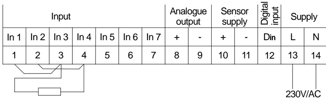
Measurement of a resistance thermometer (e.g. PT100) or resistance in the 3-wire; supply voltage 24 VAC
