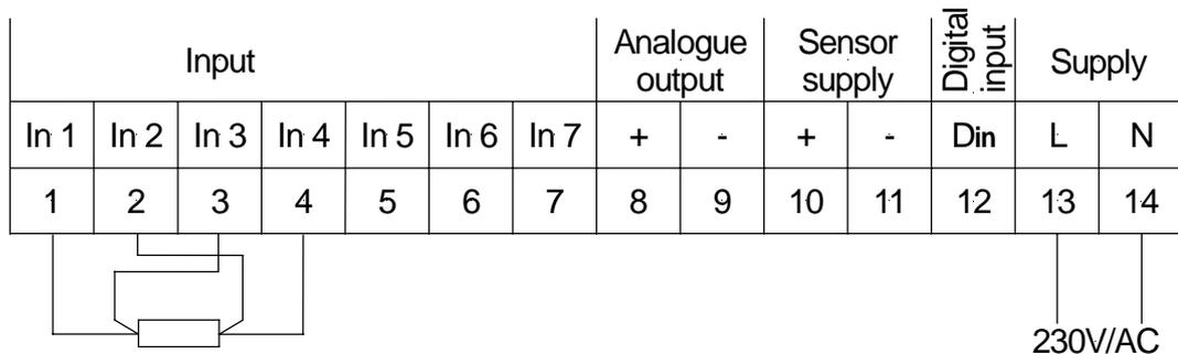
Measurement of a potentiometer in the 4-wire technology
