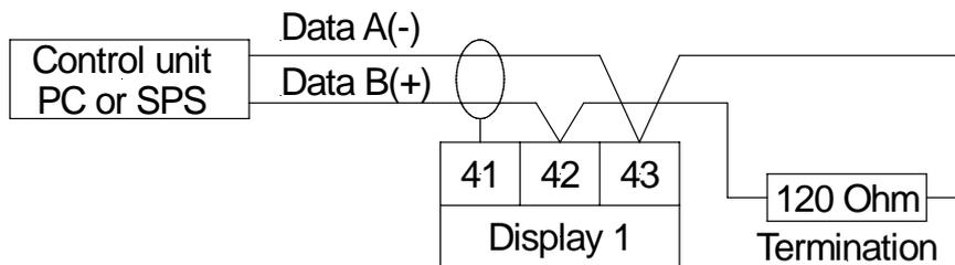
**Caution!** The potential reference can lead to a compensating current (interface  $\Leftrightarrow$  measuring input) with a non-galvanic insulated interface and can thus affect the measuring signals.
