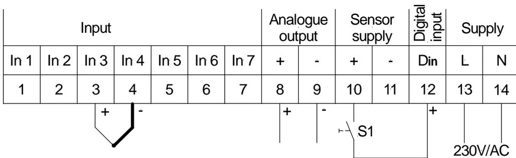
Measurement of the shunt resistance; connection to the analogue output; connection of the digital input to the sensor supply; supply voltage 230 VAC.
