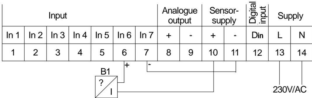
Measurement of a voltage signal (5 V or 10 V) from a 3-wire transmitter using the sensor supply; supply voltage 24 VDC
